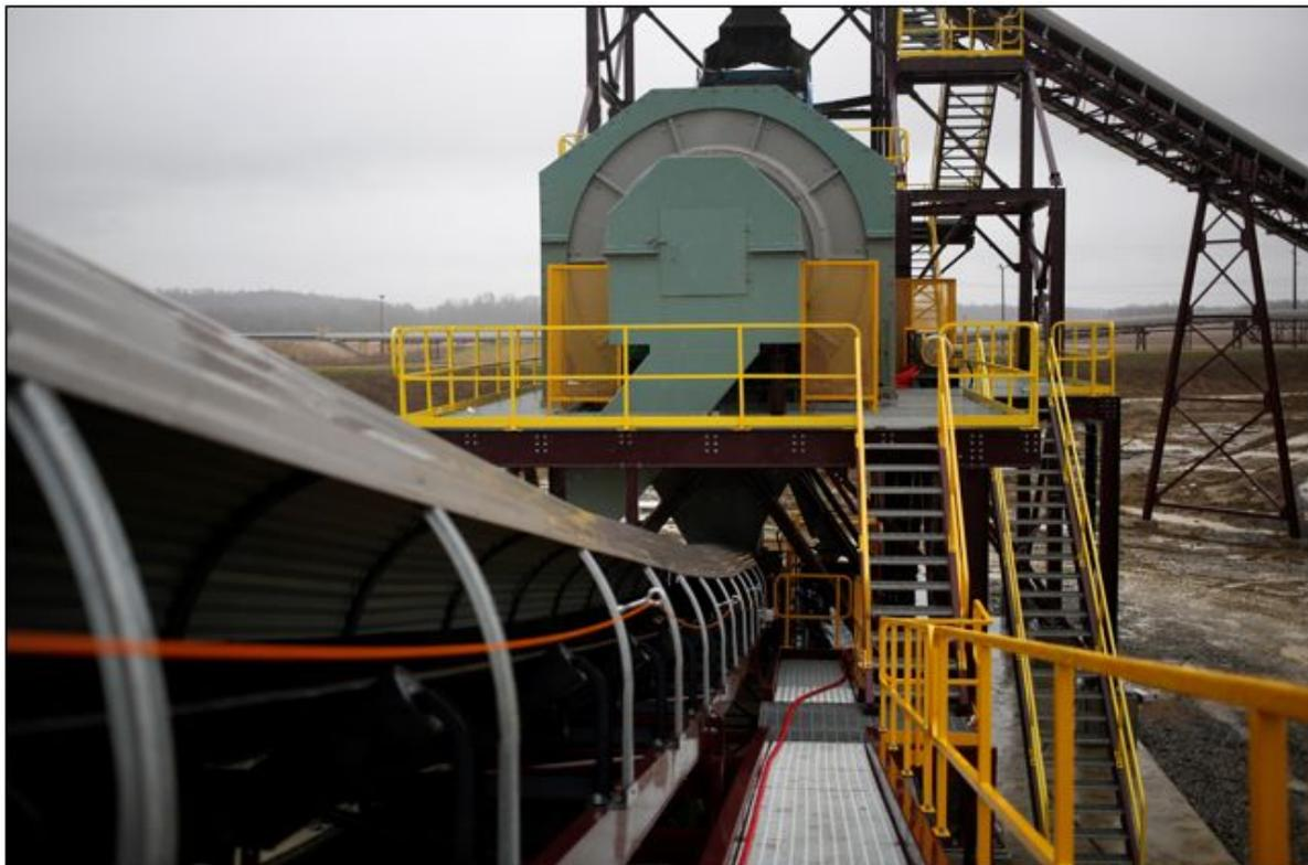
*Figure 4: Rotary breaker feeding raw coal to the Poplar Gove CHPP*
