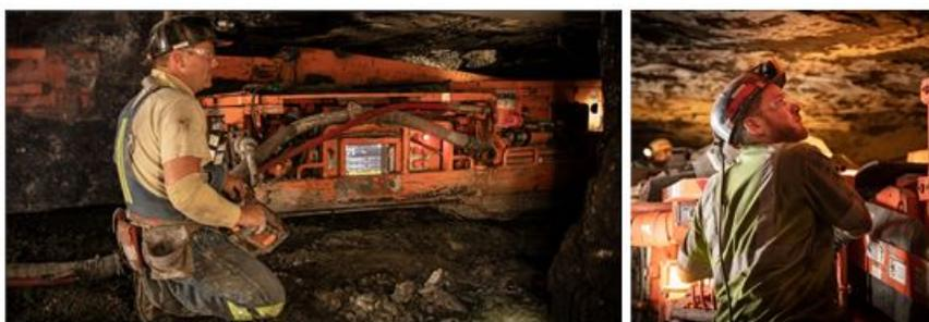
*Figure 1: Underground continuous miner & roof bolter in operation at Poplar Grove*
